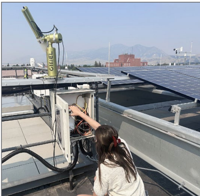
MSU graduate student Morgan Hasenmyer adjusts the AERONET solar radiometer on the MSU Bozeman campus during measurements of extremely smoky air in August 2026.
